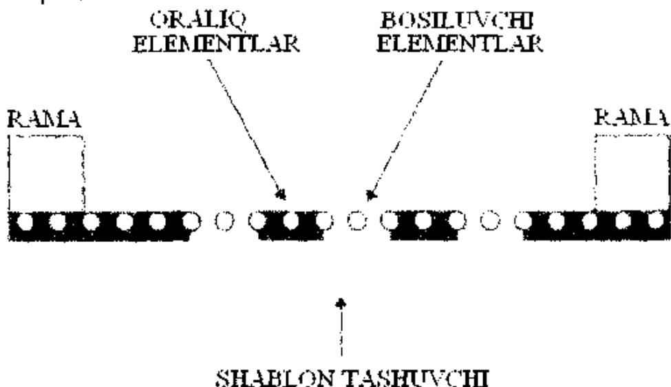
*2.6-Rasm. Trafaret bosma qolipining tuzilish prinsipi*
