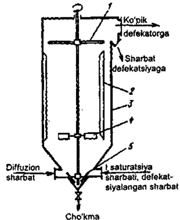
6.6-rasm. Optimal olddefekatsiyalash apparati.
