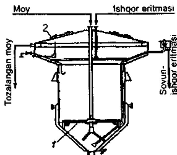
5.20-rasm. Sovun-ishqor multitida moyni neytrallashtirish apparati.
