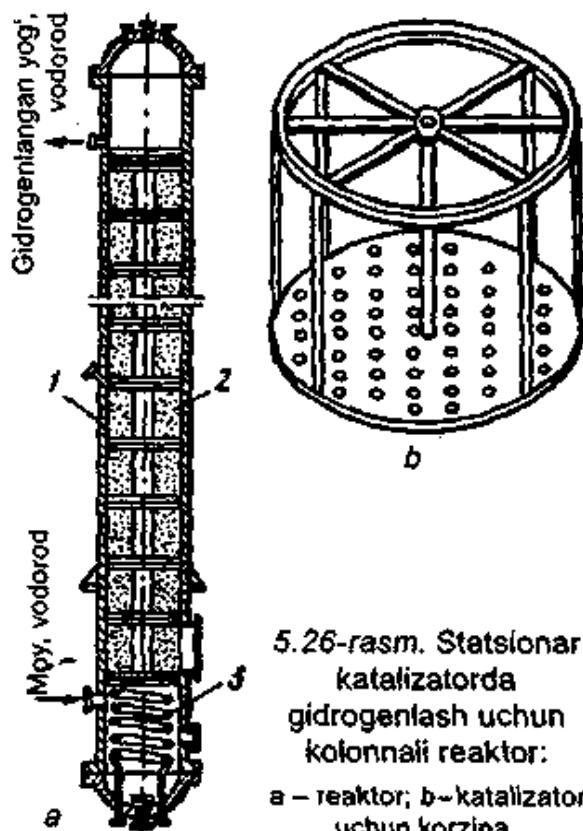
5.26-rasm. Statsionar katalizatorda gidrogenlash uchun kolonnali reaktor:
