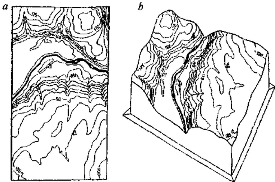
**4.5-rasm. Joyning relef kartasi (a), uning gorizontallarda avtomatik ravishda tuzilgân blok-diagrammasi (b).**
